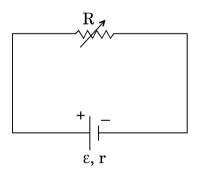
A variable resistor R is connected across a cell of emf ε and internal resistance r as shown in the figure. Draw a plot showing the variation of (i) terminal voltage V and (ii) the current I, as a function of R.
